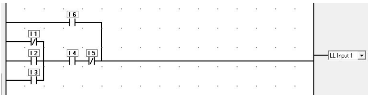
Figure 7 Multiple Logic Conditional Example
