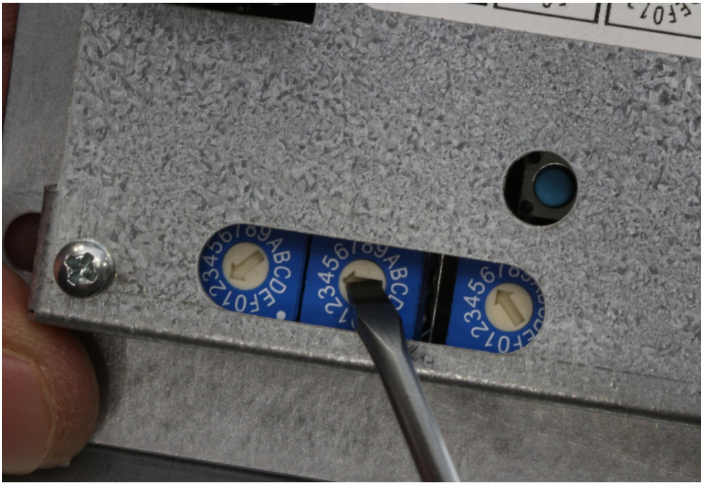
Figure 11 Setting the TSS Device Address
