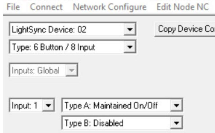
**Figure 21 - Network Link LS Input Settings**
