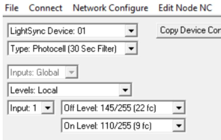
**Figure 16 - Outgoing LLNC Photo Sensor On/Off control**
