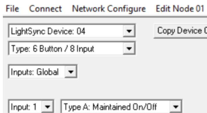
**Figure 17 - Outgoing Global Setting for On/Off Control**
