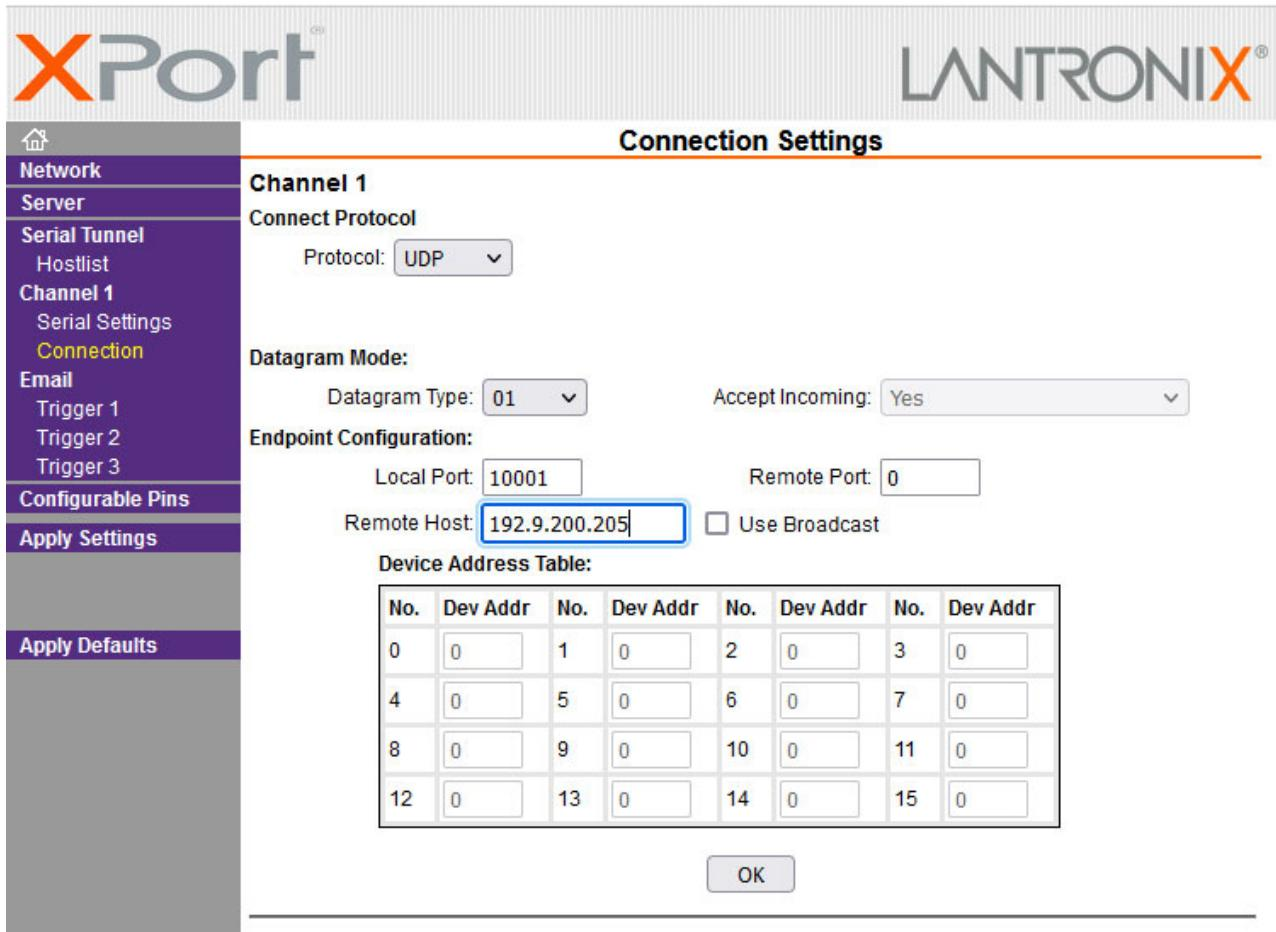
**Figure 6 - UDP Unicast Connection Screen**
