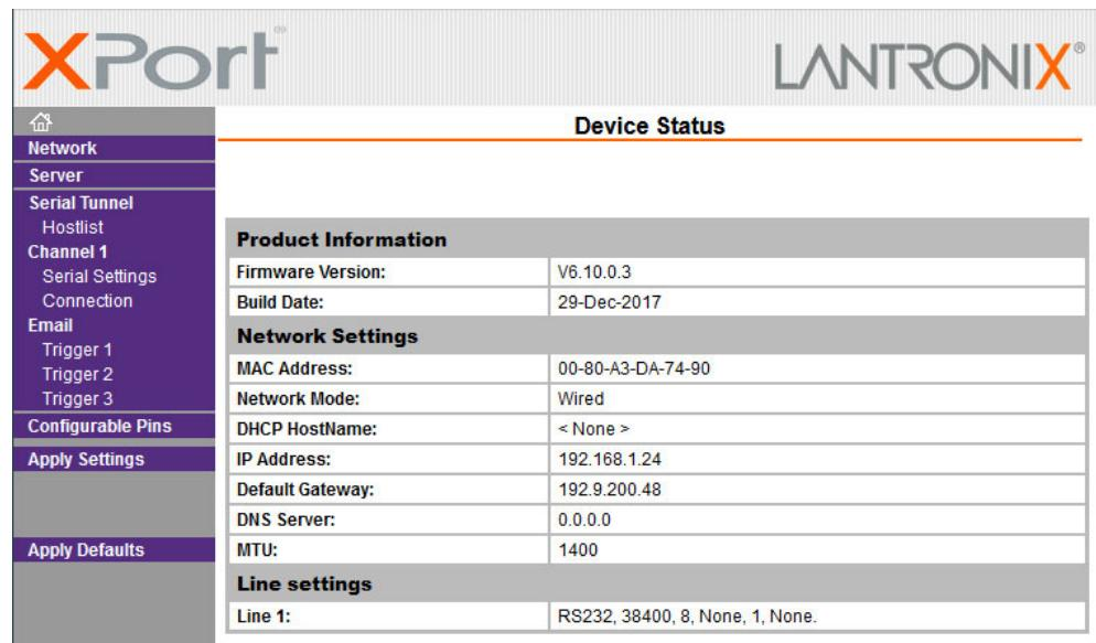
The screenshot shows the XPort Network Home Page. The left sidebar menu includes: Network, Server, Serial Tunnel, Channel 1 (Serial Settings, Connection), Email (Trigger 1, Trigger 2, Trigger 3), Configurable Pins, Apply Settings, and Apply Defaults. The main content area features a "Device Status" bar at the top. Below it is a "Product Information" section with the following details:
