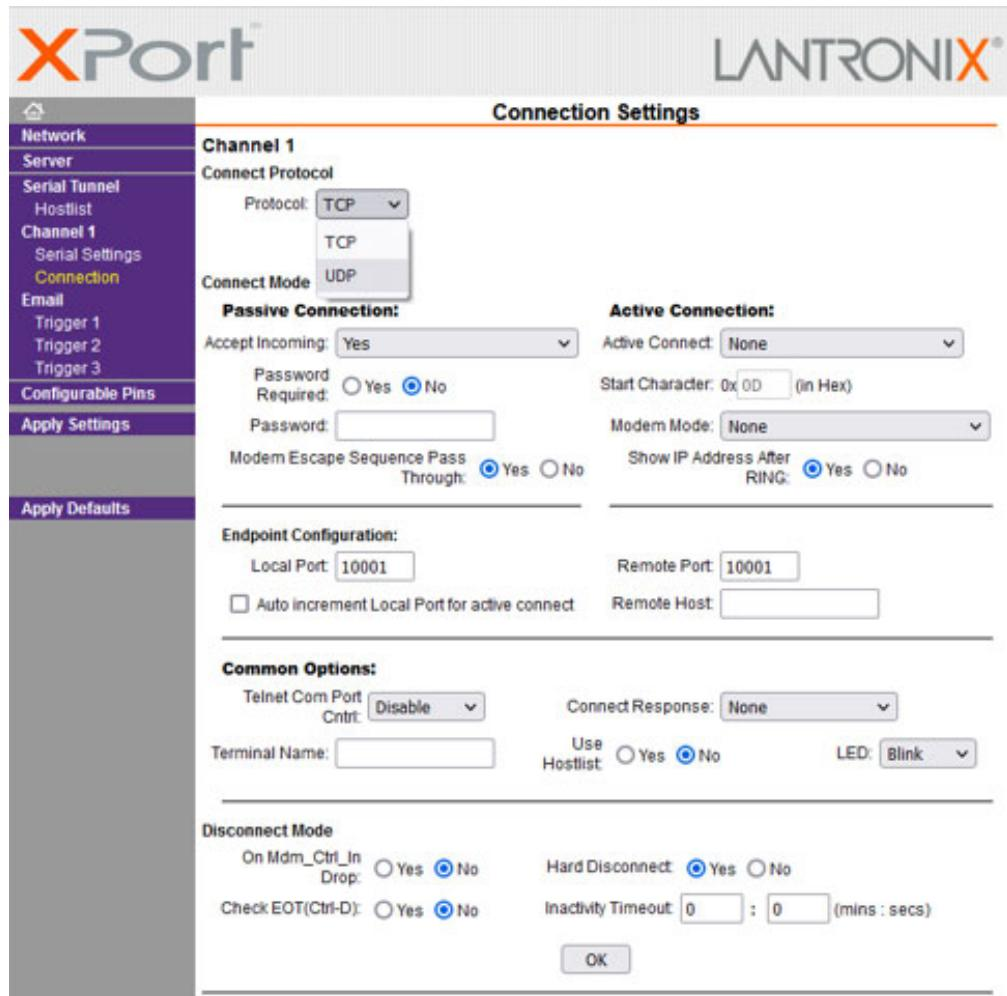
Figure 5 - Default TCP Setting Connection Screen
