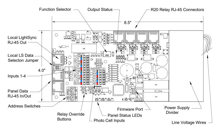
**Local LightSync:** Provides data and power connection for CAT-5 data line cable to LightSync switches and devices.
