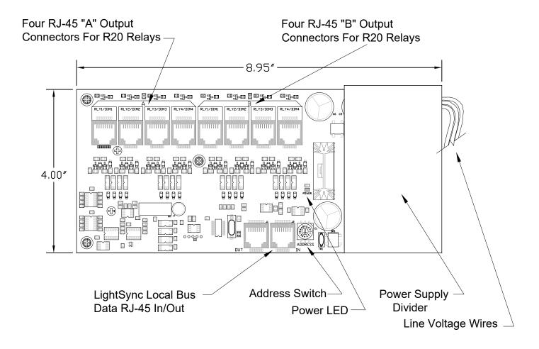
**LightSync Data In/Out:** Connection from the lightLEEDer panel "Local Bus" to provide communication to the EVO X.
