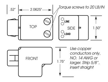
"C" designates integral connector designed for ILC I/O board relay outputs.
