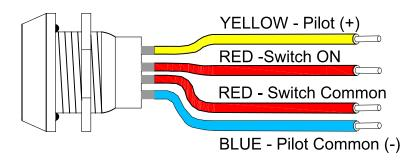
WTB Push Button Switch with LED Status Ring Momentary closure, IP65 rated with silicone rubber O-ring
