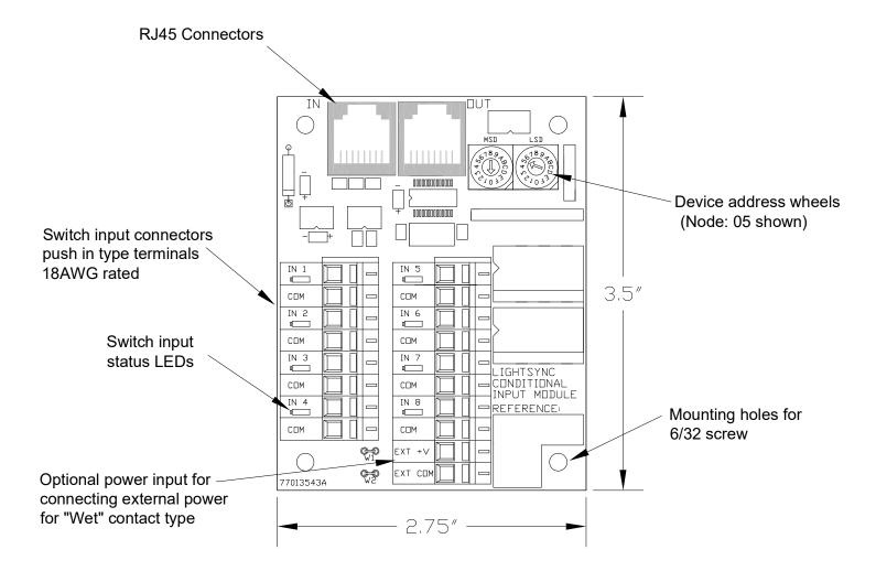
Switch inputs for dry contact closure type low voltage switches Switch closure LED status indicator Switch inputs provide power at 12VDC to the switch Inputs trigger at .05ma on a 1/2 second closure
