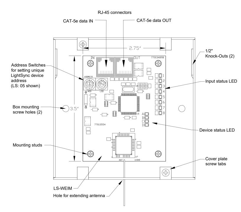
The LightSync Wireless EnOcean Input Module (LS-WEIM) is equipped with an 902MHz transceiver for communication with wireless devices within a 100' Radius.
