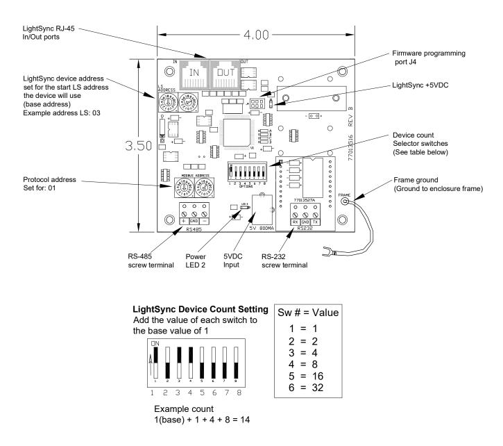
The LightSync LSSIICM RS-232/485 module is for interfacing a BAS or AV system with ASCII or ModBUS protocol. This device is a LightSync input module and is addressed in the LS network as one, or up to 64 LS devices as needed. This module supports RS-232 or RS-485 communication and receives commands from the BAS or AV system to trigger the assigned LightSync switch input points.
