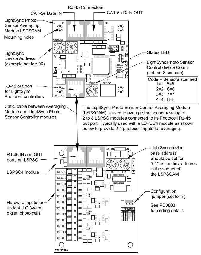
This can be used with any combination of LSPSC or LSPSC4 modules for up to 8 sensors averaged in the LSPSCAM.
