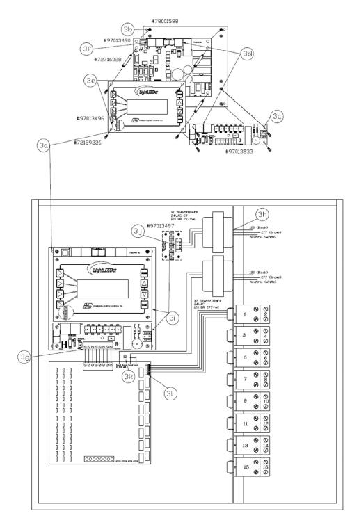
a. Install RSX to LL Backplate #78001588 to existing back plate using 4 screws provided
