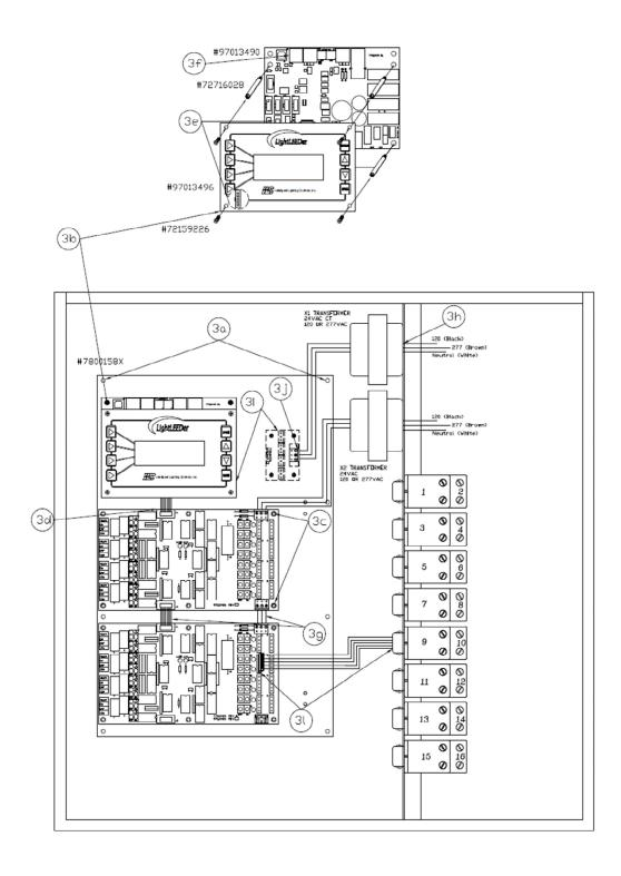
a. Install Retrofit Backplate #78001584/5/6 to existing back plate using screws provided
