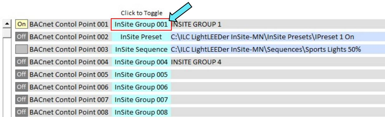
Figure 16 – Toggling the InSite Control Point Type
