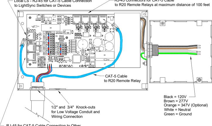
RJ-45 for CAT-5 Cable Connection to Other LightLEEDer Panels When Networked
