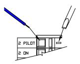
To connect wire to the input, insert a small straight blade screwdriver in slot and apply pressure to open the spring clamp, insert wire then release.
