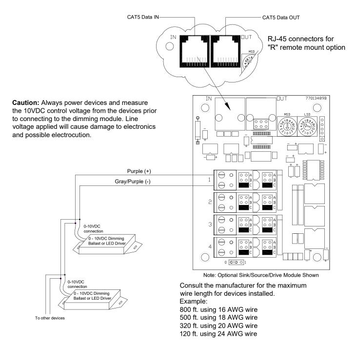
The LightSync Dimming Module provides 4 independent zones for controlling ballasts, LED drivers or other devices that have 0 - 10VDC control. Each control port can control up to 200 ballasts parallel connected based on a typical current of .5mA each, with a maximum of 100mA per output channel or dimming zone. Consult manufacture for current requirements and recommended wiring practices for class 2 wiring.
