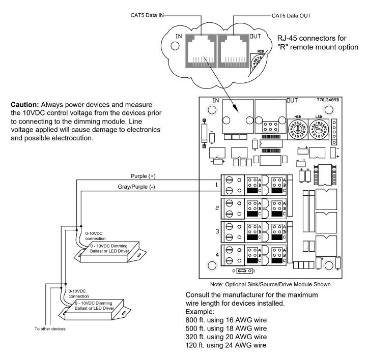
The LightSync Dimming Module provides 4 independent zones for controlling ballasts, LED drivers or other devices that have 0 - 10VDC control. Each control port can control up to 200 ballasts parallel connected based on a typical current of .5mA each, with a maximum of 100mA per output channel or dimming zone. Consult manufacture for current requirements and recommended wiring practices for class 2 wiring.
