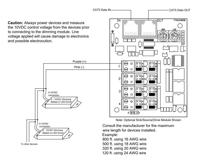
The LightSync Isolated Dimming Module provides 4 independent zones for controlling ballasts, LED drivers or other devices that have 0 - 10VDC control. Each control port can control up to 200 ballasts parallel connected based on a typical current of .5mA each, with a maximum of 100mA per output channel or dimming zone. Consult manufacture for current requirements and recommended wiring practices for class 2 wiring.
