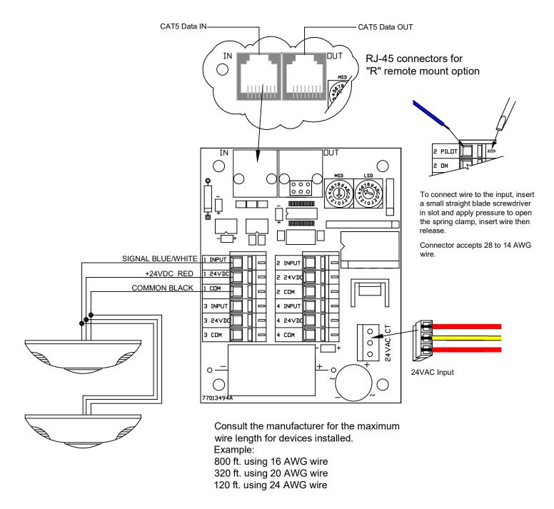
The LightSync Occupancy Sensor Input Module provides power and receives signals from sensors on each of its 4 independent inputs. The module provides up to 200mA @ 24VDC to power the sensors and accepts the 24VDC signal directly at the input.
