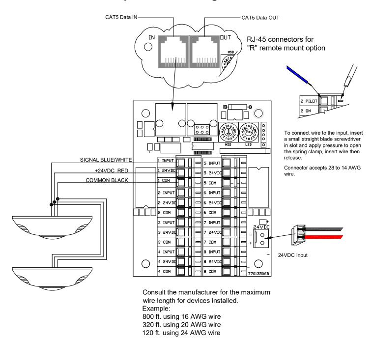
The LightSync Occupancy Sensor 8 Input Module provides power and receives signals from sensors on each of its 8 independent inputs. The module provides up to 800mA @ 24VDC to power the sensors and accepts the 24VDC signal directly at the input.
