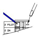
To connect wire to the input, insert a small straight blade screwdriver in slot and apply pressure to open the spring clamp, insert wire then release.
