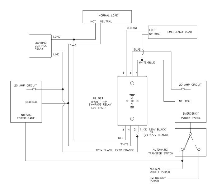
This is a typical wiring diagram for a lighting control panel that is controlling normal loads and emergency loads simultaneously. This is accomplished by signaling the Emergency Power Control unit (EPC-1) from the lighting controller. With the use of an EPC-1 during normal conditions, the relay panel controls the normal loads and signals the EPC-1 to control the emergency loads. During a power outage, the EPC-1 by-passes the normal load and illuminates the emergency lighting loads only.
