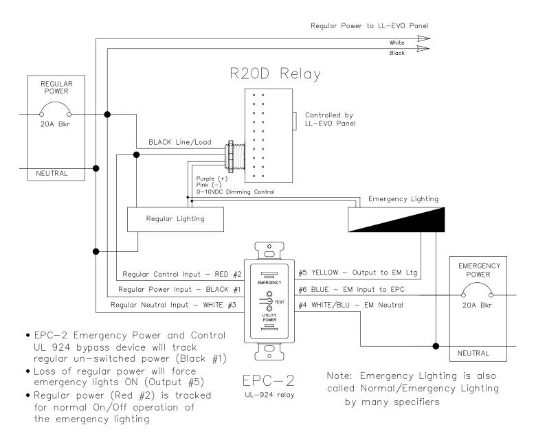
Note: Normal power to R20D relay, LL—EVO controller, and EPC—2 must be on the same circuit for the 0—10V dimming bypass operation to function properly.
