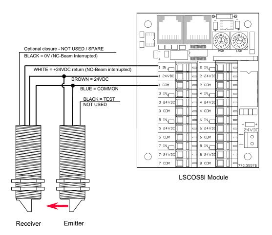
Photoelectric Partition Sensor wiring to LightSync conditional occupancy sensor input module for disabling ILC "Echo" inputs when wall partition is out and beam is interrupted - use white return wire (no). optional black (nc) return should be pulled to input module for reverse wiring if needed.
