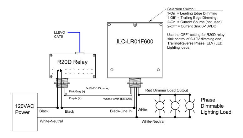
The ILC-LR01F600 selectable phase dimmer can be operated by the R20D relay for positive power off and 0-10VDC dimming control. This dimmer has a field settable switch for selecting trailing (ELV) or leading edge dimming.
