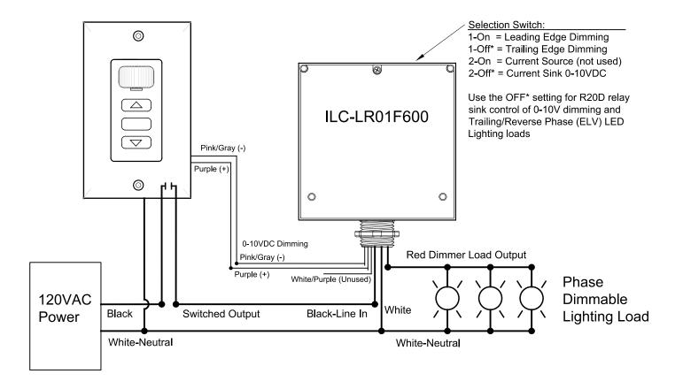
The ILC-LR01F600 selectable phase dimmer can be operated by a 0-10VDC dimmer switch with on/off power control. This dimmer has a field settable switch for selecting trailing (ELV) or leading edge dimming.
